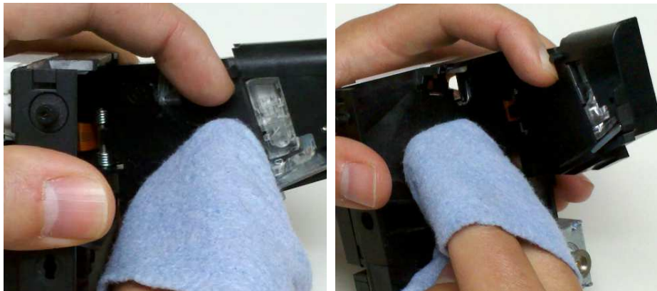
Fig. 3: Cleaning the coin flap and rail of EMP 800v6 with a soft tool
